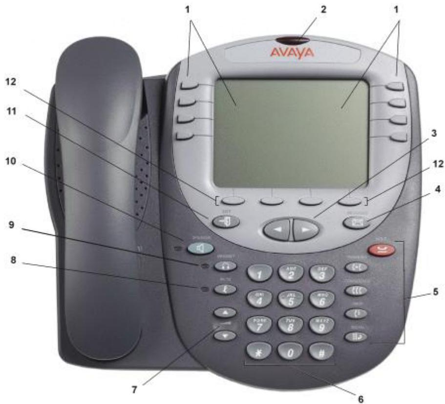
1. **Display, Call Appearance and Feature buttons:** Call Appearance Keys allow the user to handle multiple calls and the display shows call information. Details on system features (allocated by your System Administrator) can also be displayed.
